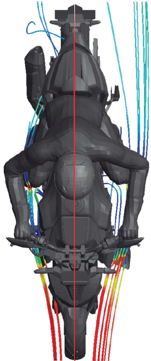
Due to its angles and frontal surface, it creates an overpressure on the top of the spoiler. The turbulence create below, generates a difference of pressure between the upper and lower part of the spoiler. Which ultimately generates the aerodynamic downforce.
